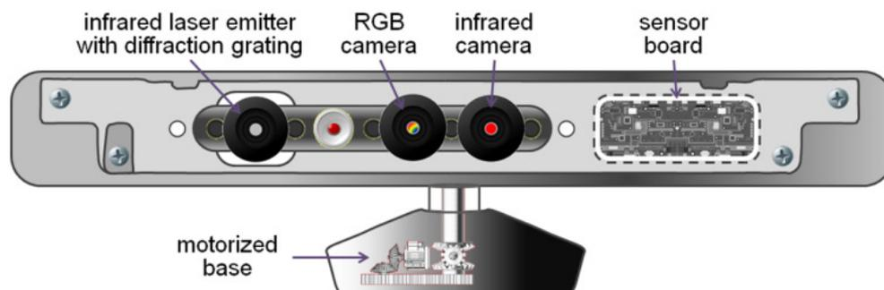
Figure 1: Schematic view of the Microsoft Kinect™ RGB-depth camera implemented for ergonomics analyses.
