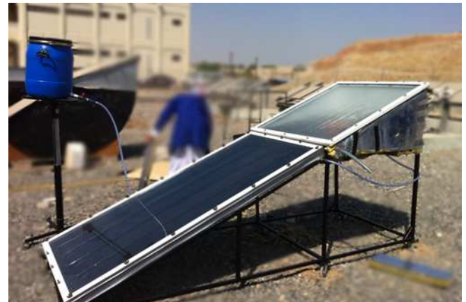
Fig. 1 Experimental set up of single slope solar water still with solar energy heating system
