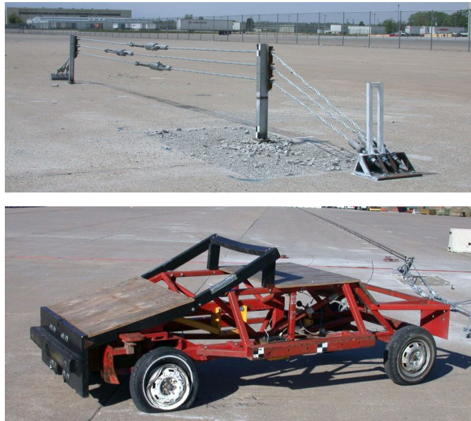
Figure 2. CTB-4, Prototype End Terminal and Bogie Vehicle
