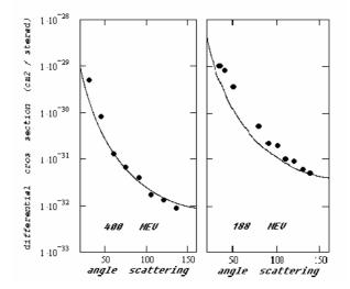
Figure 2: Comparison of the calculated effective scattering crosssections of electrons with energies of 400 and 188 MeV (the continuous curve) with the experimental data (points) taken from [9].
