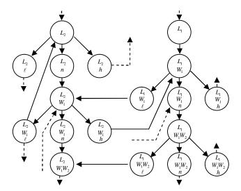
Fig 2. A part of transition system model of N-M switching control system.
