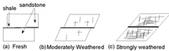
Fig. 12 Deformation model of the alternative layers of sandstone and shale at different weathering degrees
