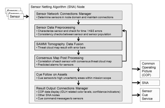
Figure 1. Prototype SNA process block diagram showing key components, input streams, and outputs.
