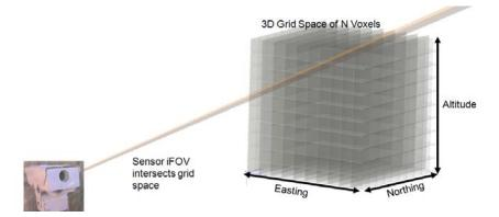
Figure 5. A standoff sensor path integrated measurement is shown passing through a UTM coordinate grid space. The standoff sensor's iFOV is shown as an elongated pyramid shape for a rectangular detector element.
