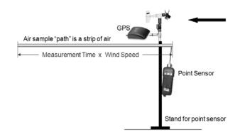
Figure 3. Point sensor measurements are converted to path integrated concentration (CL) line segment vectors using the wind velocity and sensor integration time. In an actual sensor network, the local wind velocity for a given point sensor may be estimated using a MET model and a network of a few wind sensors. A cross sectional area "domain" (e.g.,  $1 m^2$ ), which is analogous to a standoff sensor instantaneous field of view (iFOV), must be assumed for the point sensor line segment vector.
