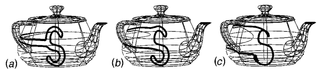
Fig. 10 Multiresolution editing without constraints is shown for the curve on the body of the Utah teapot in Fig. 9. Three resolution levels of a single select-and-drag operation and no constraints are shown.
