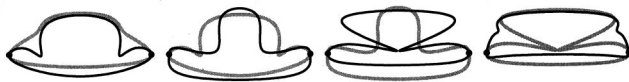
Fig. 7 A Y-symmetric curve with a constant area has a positional constraint on the left and a tangential constraint on the right. Several direct manipulation operations are performed while, effectively, these two constraints keep the curve at a constant width, throughout. The previous operation is shown in gray and the new one is shown in black, from left to right. These examples were created in a few seconds.
