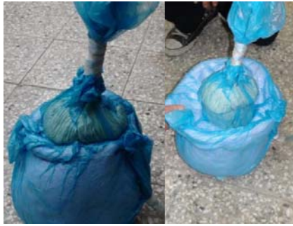
Fig. 7 The positive sand mould was sucked to form the stump shape
