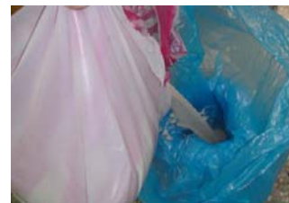
Fig. 8 The plastic bag was filled with sand to form a positive mould
