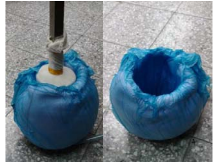
Fig. 6 The negative mould was vacuuming(left), and the stump was pulled out (right)
