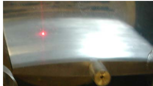
Figure 2 : Portable digital vibrometer setup for hydrofoil vibration measurements
