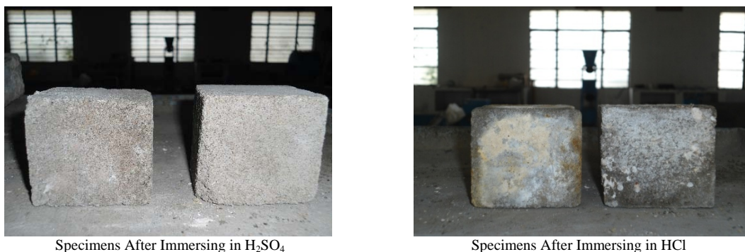
Fig 1 Specimens after immersing in Acids after 14 weeks
