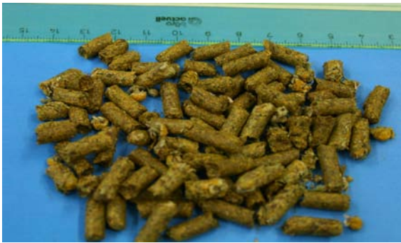
Fig. 3. Pelletized chamomile plant material (raw material for the fluidized bed extraction)
