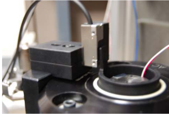
Figure 6. Optical encoder read-head sensor and read-strip optical scale mounted on Model 394A30 calibration air-bearing shaker.
