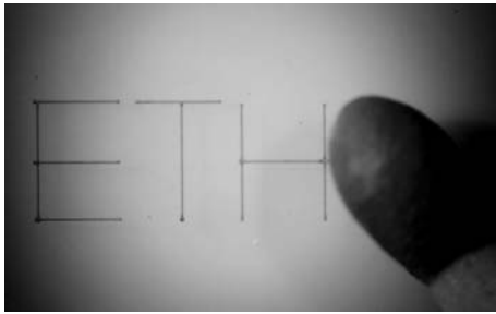
Fig. 1 Printed and cured ETH Logo compared with the head of a match. The width of the lines is 62 \mu\text{m} .
