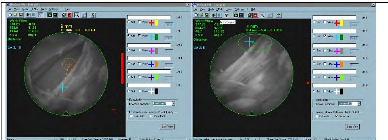
Figure 8: Coagulation support for the case of a red out situation. The shown grey level images are previously stored images corresponding to the current position. Left: The orange graphic overlay of the coagulation fibre is far away from the coagulation point (blue mark). The red alarm signal on the side shows that the 3D distance is large. Right: The coagulation fibre has been brought into the correct depth and right x-y-location, the red alarm signal is low. Coagulation was successful and the bleeding stopped.
