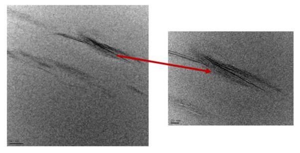
Figure 3. TEM images of P2 nanocomposite at different magnifications. Dark lines representing clay layers.
