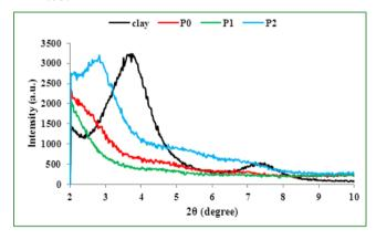
**Figure 1.** XRD traces of organoclay (Closite20A) [11], and the studied nanocomposites: P0 [11], P1 and P2.
