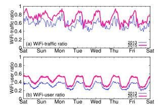
Figure 6: (a) WiFi-traffic ratio and (b) WiFi-user ratio.
