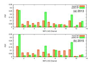
Figure 16: Associated 2.4GHz channels (2013 and 2015).
