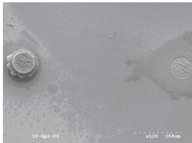
Figure 3. SEM picture of a sheared off substrate.
