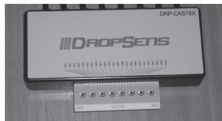
FIGURE 1: Details of biosensor device used for measuring cell-pesticide interactions. The eight-channel disposable sensor is connected to the potentiometer through a customized interface.
