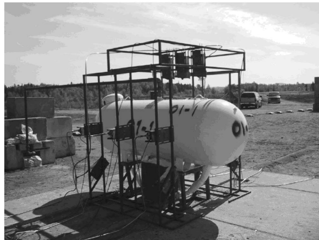
Fig. 2 1.9 M 3 tank with burners (2001 tests with three vapor space burners and ten liquid space burners)
