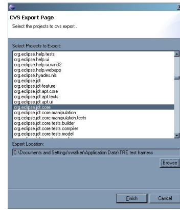
Figure 1: The Eclipse wizard used to select CVS projects for extracting change history data. Here, change history data is about to be extracted from the org.eclipse.jdt.core project.
