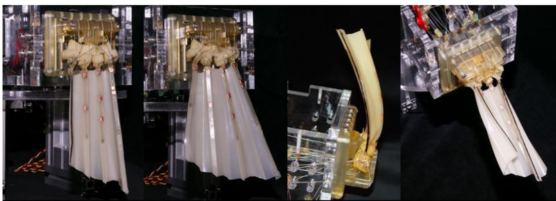
Figure 2: Component motions: from left to right, fin relaxed, expanded, curled, and cupped.
