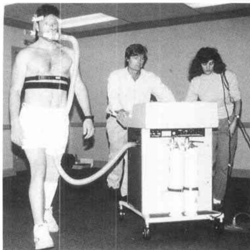
Fig. 2. Subject ambulating while being tested with MMC Horizon Metabolic Cart and Vantage Heart Rate Monitor.
