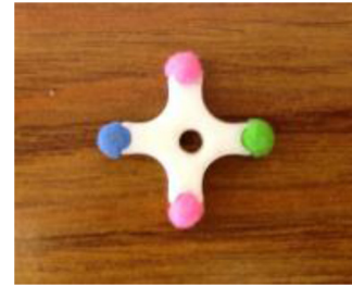
Fig. 1 Four colored markers mounted on the surgical tool
