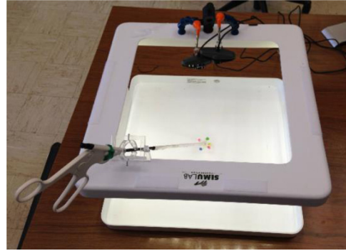
Fig. 5 Prototype of laparoscopic training system with cameras
