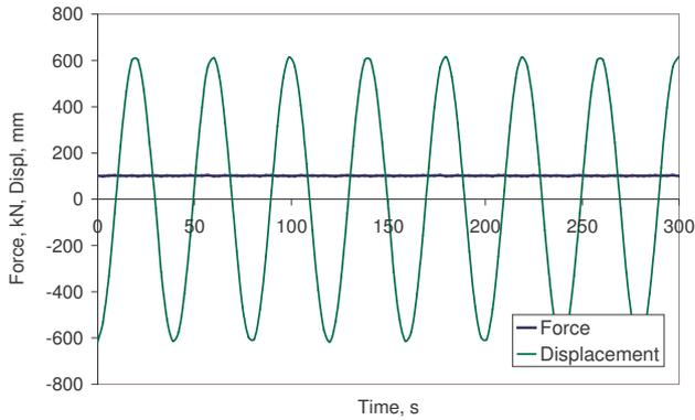
**Figure 17. Load and displacement of handling rope sample during BOS tests**
