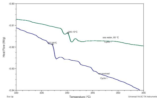
**Figure 6. Glass transitions of Twaron1000 fibers: lower, as received, upper, after 231 days in sea water at 80 °C.**
