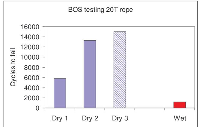
**Figure 18. 20T handling rope on sheave and bend over sheave results.**
