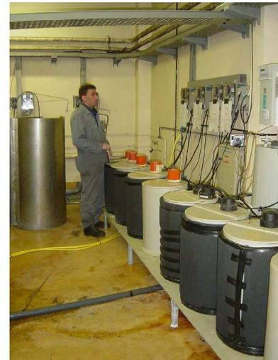
**Figure 2: Temperature controlled circulating sea water and pure water tanks**
