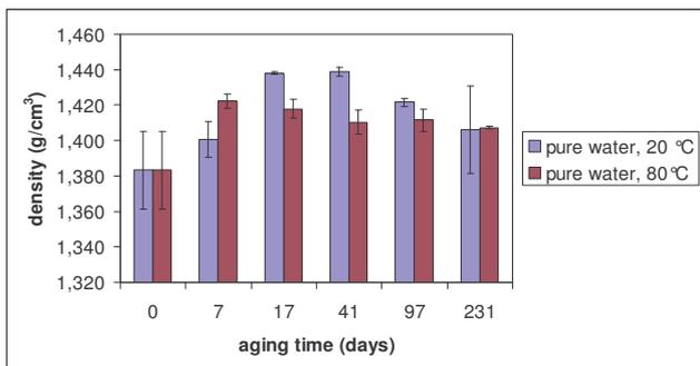
**Figure 5: Density versus aging time of Twaron 1000 fibers immersed in pure water at 20 and 80 °C**
