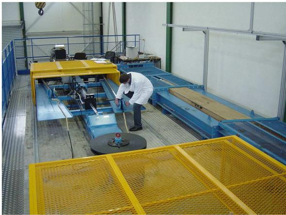
**Figure 14. Bend-over-sheaves test machine specifically designed to test ropes on full size oceanographic sheaves up to 2 meter diameter.**
