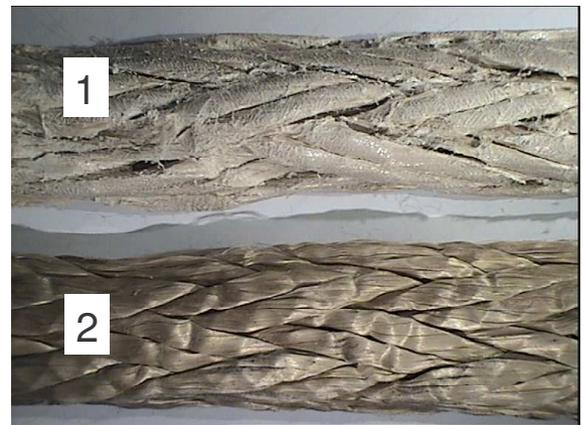
**Figure 16. New and used rope after 7 years service, appearance with cover removed.**
