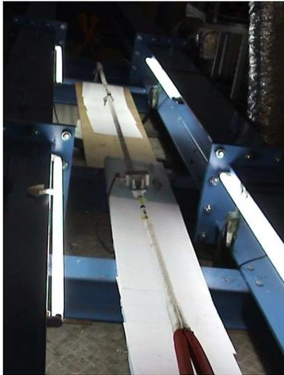
**Figure 13. 20T break load *Twaron 1000* aramid rope on 100 ton capacity test frame during strain calibration trials.**
