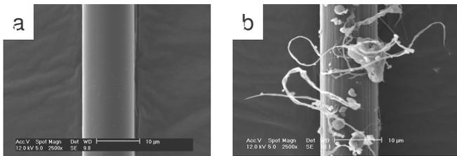
Figure 8: SEM photos of *Twaron 1000* fibers (a) as-received, (b) after 231 days in sea water at 80°C
