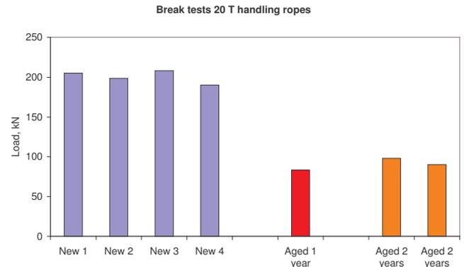
**Figure 15. Strength retention, handling ropes**
