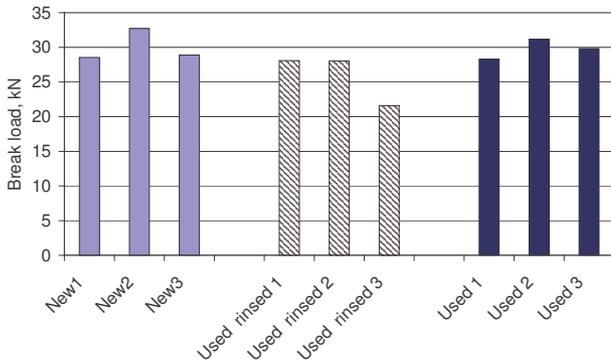
**Figure 11. Tensile test on aramid instrumentation line samples new and after use. Upper, test set-up showing cone termination, lower, test results.**
