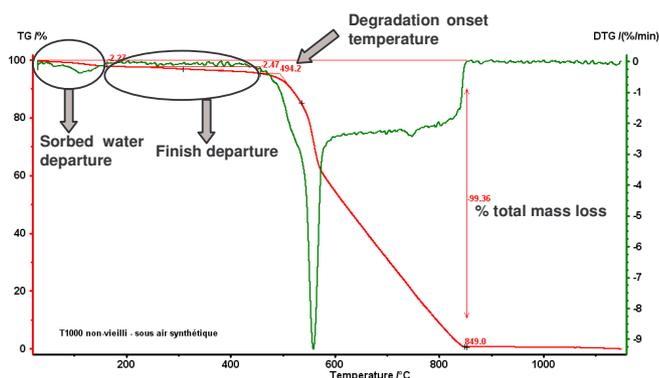
**Figure 7: Profile and interpretations of thermogram obtained from as-received Twaron 1000 fibers**
