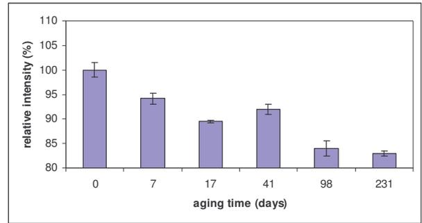
**Figure 4: Relative intensity change of the peak related to the finish for *Twaron 1000* fibers, pure water, 80°C.**
