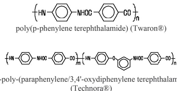
Figure 1. Aramid molecular structures
