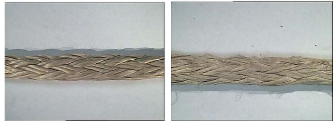
**Figure 19. Sections taken from wet handling rope after BOS test
