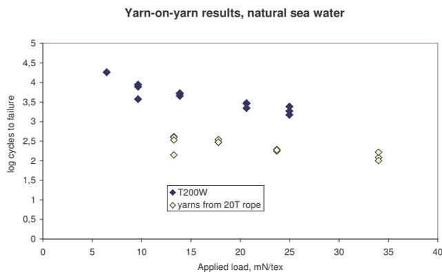
Figure 20. Yarn-on-yarn abrasion test results.
