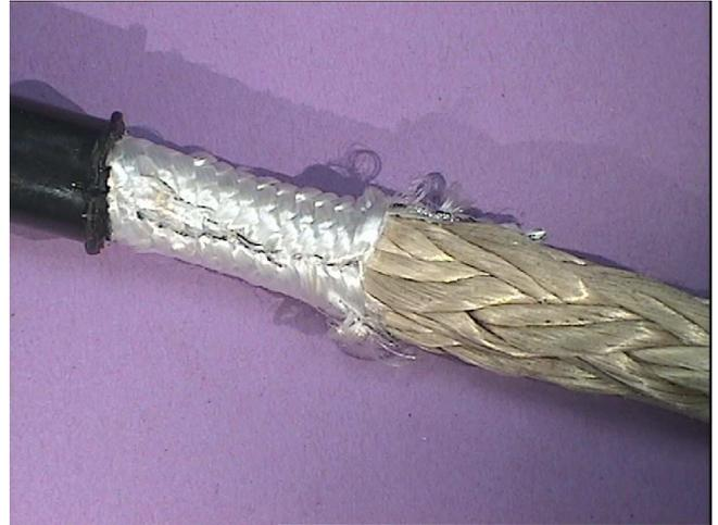
**Figure 12. Handling rope construction showing from left to right elastomer cover, polyester braid and aramid core.**
