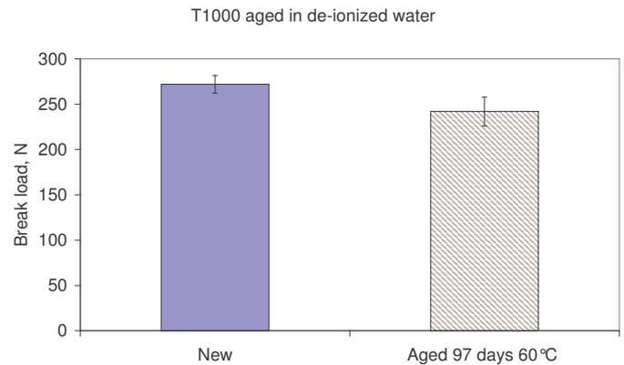
Figure 9. Tensile tests on *Twaron 1000*, 8 samples of new and aged yarns.
