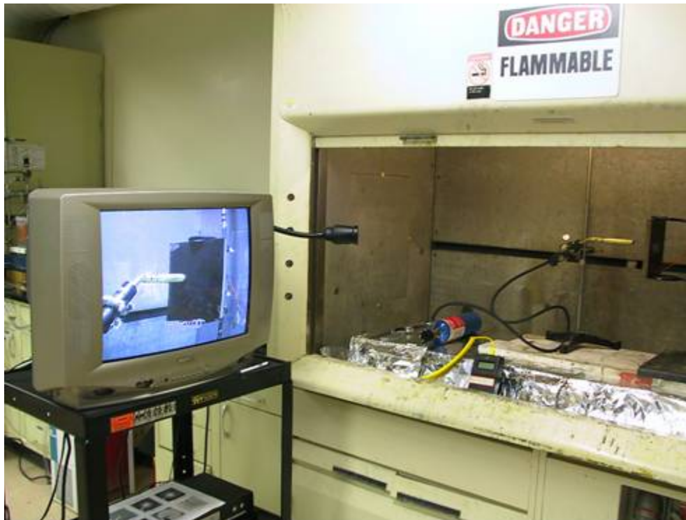
Figure 1 Photograph of fire test setup showing video camera, propane torch and test coupon
