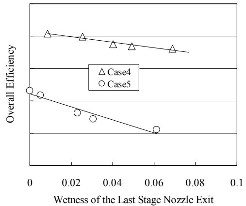
Figure 7 Overall efficiency with various wetness and back pressure in the 48'' LP turbine
