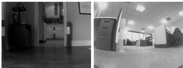
Fig. 5. Example images from the SEQ2 (left) and SEQ3 (right). The reflector beacons are NAV200 fiducials used for ground truth estimation
