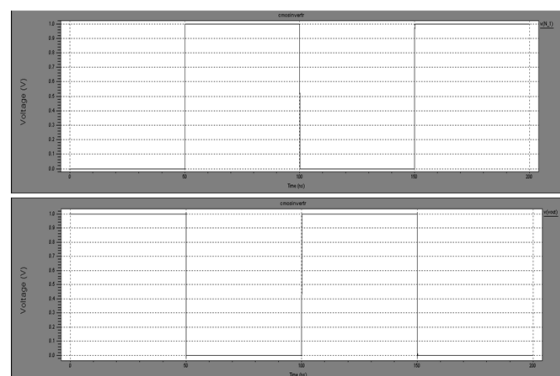
Fig 2 Input and Output Waveform for NOT Gate
