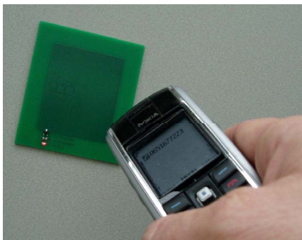
Fig. 10 Rectenna feeding a LED. Wirelessly powered by a GSM-1800 mobile phone, transmitting at a peak-power level of 1W .
