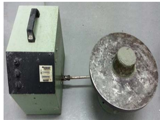
Fig. 2. Set-up of the flow table test.
