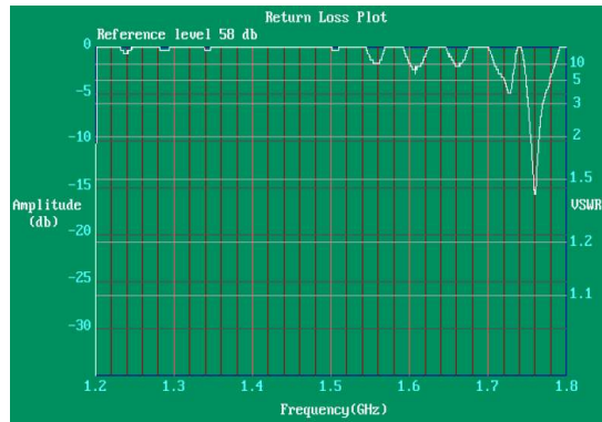
Fig. 5. Measured return loss of SCTSP_E2.
