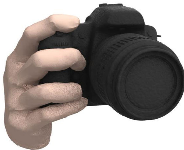
Figure 1. An example of ergonomic assessment by integrating the digital hand model with the 3D product model of a digital camera
