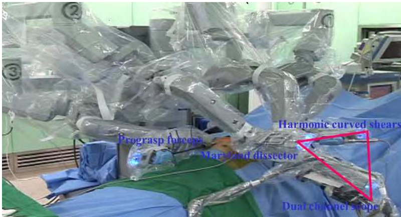
Fig. 6. Following the insertion of all robotic instruments through the axillary and anterior chest skin incisions, the three external joints of the robotic arms should form an inverted triangle.
