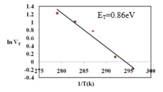
Figure 7. The activation energies for bulk (E<sub>T</sub>) etch rate for alpha +laser
