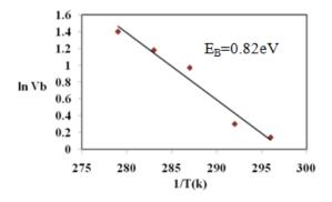
Figure 2. The activation energies for bulk (E<sub>B</sub>) etch rate for alpha
