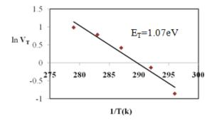
**Figure 5.** The activation energies for bulk  $(E_T)$  etch rate for alpha
