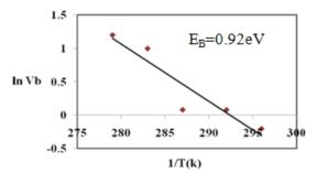
Figure 4 The activation energies for bulk (E<sub>B</sub>) etch rate for alpha + laser
