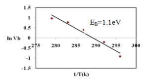
Figure 3. The activation energies for bulk (E<sub>B</sub>) etch rate for laser+alpha
