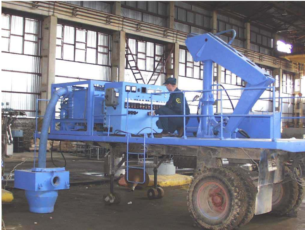
Fig.4. Mobile modular type facility to immobilise SRS in borehole type repositories.
