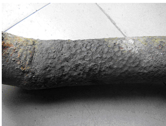
Fig. 6 Corrosion of steel pipe
