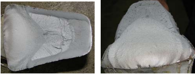
Figure 16 and 17 – The Details about the KS12 hook fracture.
