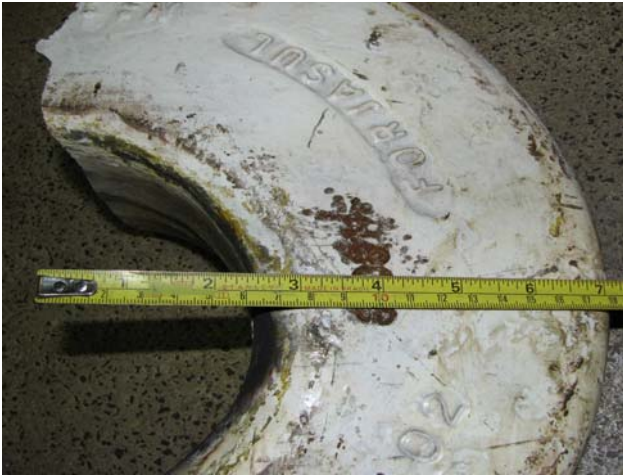
Figure 19 – The Position of KS12 hook fracture
