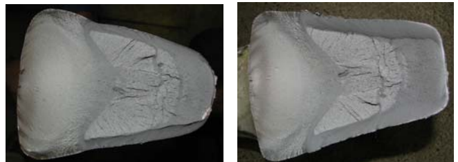
Figure 14 and 15 – The Details about the KS12 hook fracture.
