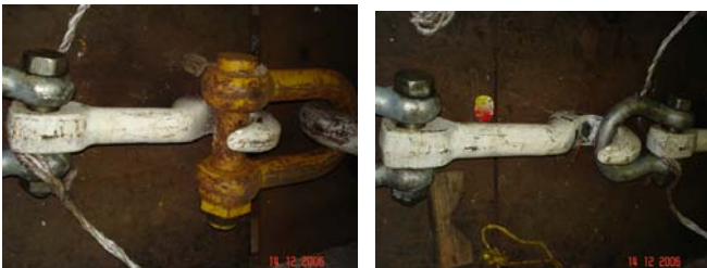
Figures 10 and 11 – KS12 Hook with and shackles and chain links connection Details
