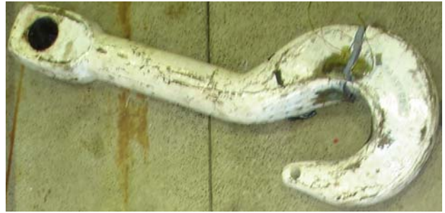
Figure 20 – The Details about the second KS12 hook fracture.
