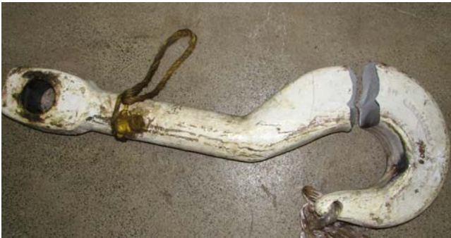
Figure 18 – The General Details about the KS12 hook fracture.
