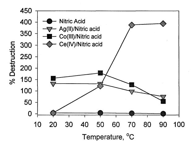
Figure 1. Percent destruction efficiency of cation exchange resin in 6.0 M nitric acid.
