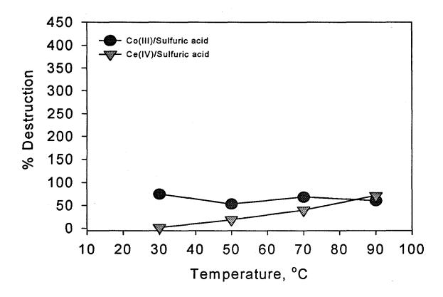
Figure 2. Percent destruction efficiency of cation exchange resin in 5.8 M sulfuric acid.
