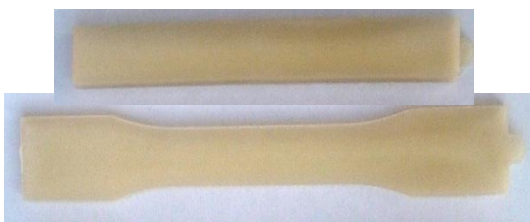
Fig 1b. Injection molded specimens for flexural creep testing
