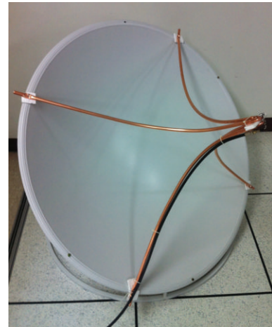
FIGURE 7: A fabricated TEM-wire fed parabola. Four ends of the TEM-wire horn are terminated by 150\ \Omega resistors to minimize return losses below 1 GHz.
