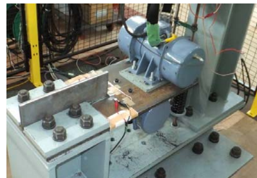
Fig. 10 The PBV-type testing machine with additional vibrator used in the springing superimposed wave loading tests.
