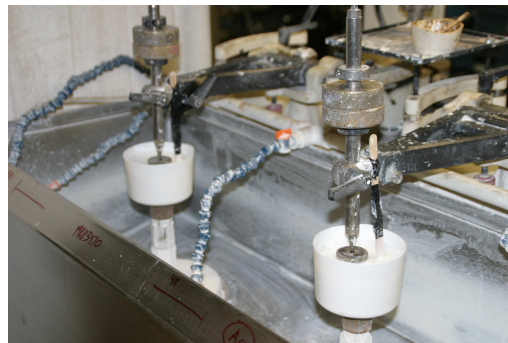
Figure 3: Photograph of the polishing test set-up
