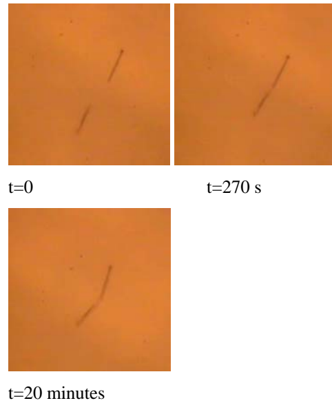
Figure 4. Attraction between two floating rod. The parameters are the same as in Figure 3. Initially, the rods are approximately parallel with their flat ends facing each other. As the rods come closer, they align so that they are approximately parallel to the line joining their centers. They maintain this orientation until touching, but after touching they rotate and are no longer parallel.
