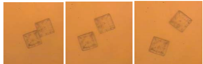
(a) 0 volts, (b) 2000 volts, (c) 4000 volts
