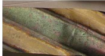
Fig 2. Examples of \text{Cu}_2\text{S} deposition on wrapping paper showing large difference in amount of deposition on the two sides of the conductor.
