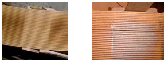
Fig.3. Examples of deposition between spacers left, and under spacer right
