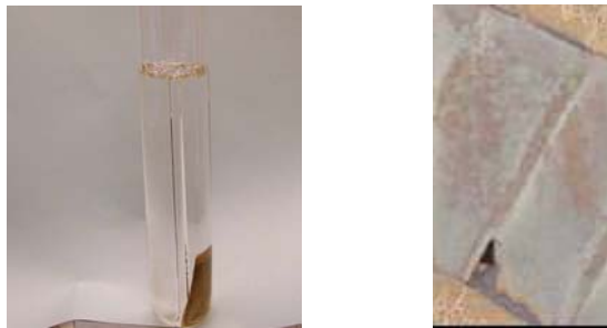
Fig 4. Laboratory experimental arrangement for Covered Conductor Deposition (CCD) test, and examples of Cu 2 S deposition on Kraft paper
