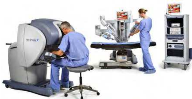
Figure 1. da Vinci system®. It consists of a surgeon's console, a patient-side cart with three or four interactive robotic arms, a high-performance InSite ® Vision System and proprietary EndoWrist ® Instruments
