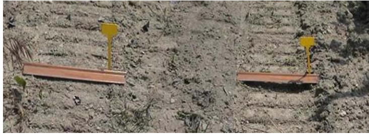
Fig. 1. Surface deformation caused by crawler tracks across the vineyard slope. Left side: upper track; right side: lower track.
