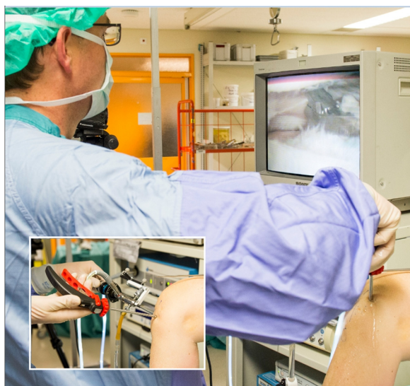
Fig. 7 Steerable cutter prototype used inside the knee by a surgeon. The photographs show that the menisci can be reached and that the prototype allows control in various grip configurations.
