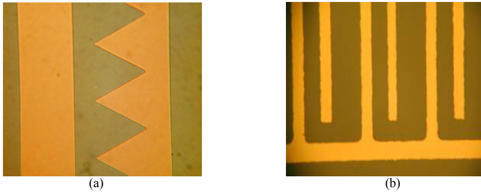
Fig. 7 Example of micro electrodes that have been fabricated in the micro fabrication at the University of Maryland at College Park: (a) saw-tooth emitter and plain collector separated by 25 \mu\text{m} ; (b) plain emitter and collectors separated by 50 \mu\text{m} .
