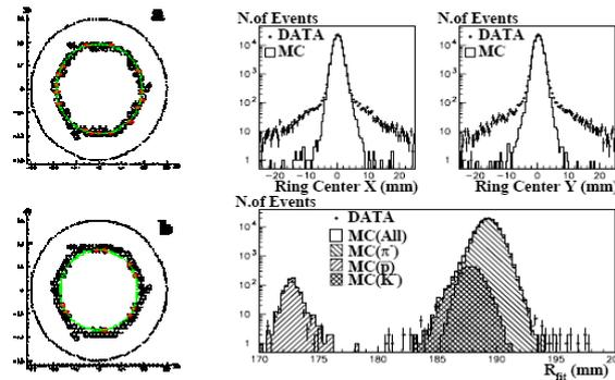
Figure 1: RICH-100 prototype performance. *Left*: the ring image for pions (a) and protons (b). *Right*: fitted ring centre (top) and radius (bottom) for different particles.
