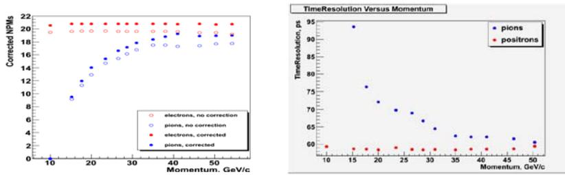
Figure 3: RICH-400 prototype, preliminary results. *Left*: number of photomultiplier hits per event as a function of momentum for pions (blue) and positrons, uncorrected (circles) and corrected (full dots) for acceptance. *Right*: time resolution vs momentum for pions (blue) and positrons (red).
