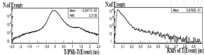
Figure 2: RICH-100 prototype time resolution. *Left*: difference between each photomultiplier time and the event time. *Right*: RMS of the average event time (right).
