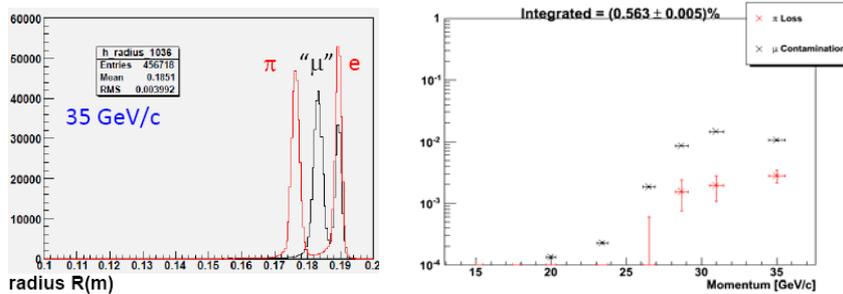
Figure 4: RICH-400 prototype, preliminary results. *Left*:  $\pi$ - $\mu$  separation at 35 GeV/c (see text). *Right*: pion loss (red) and muon contamination (black) vs momentum (mirror centered on beam line).
